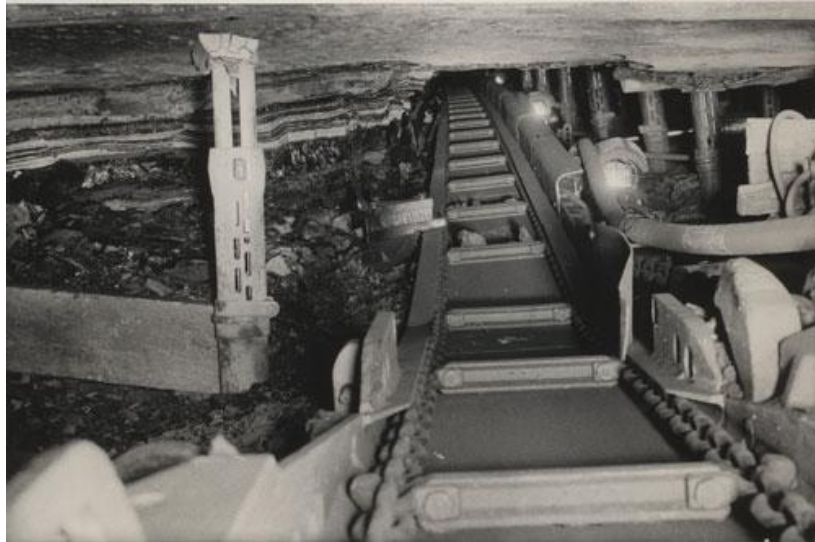
Reisshakenhobelbau in 6m3, Flöz 23, 4.10.1960
